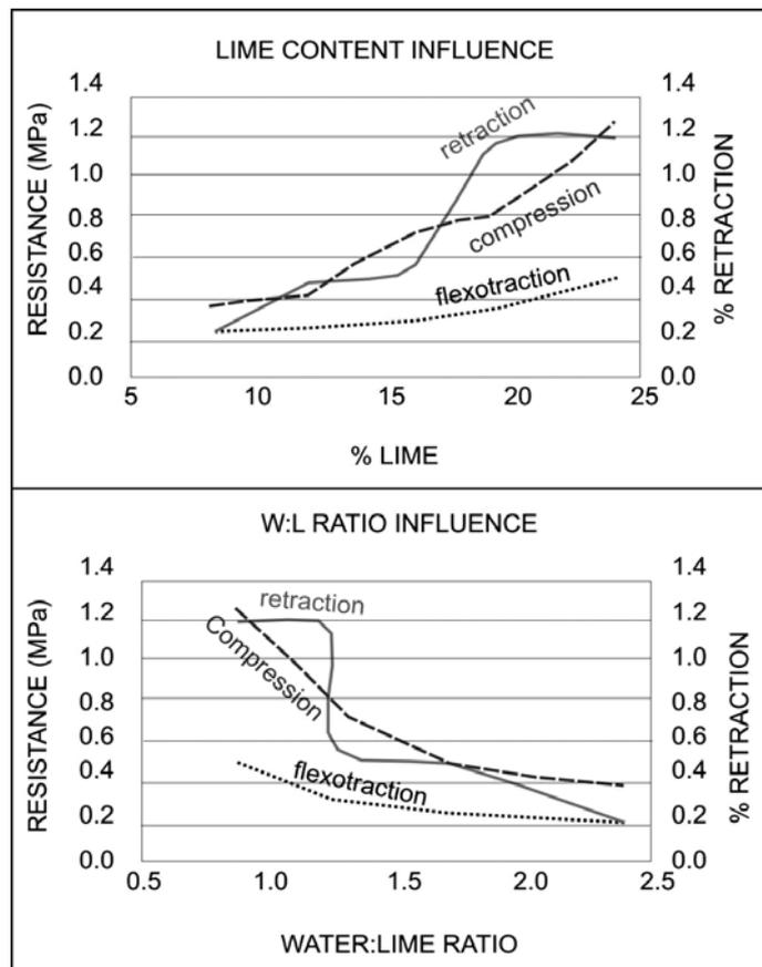
Fig. 10 - Lime content and water/lime ratio influence according to the % resistance and % retraction after 28 days.
